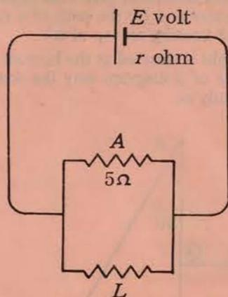
The coil  $A$  has a resistance of 5 ohm and is connected to the terminals of a cell of constant e.m.f.  $E$  volt and internal resistance  $r$  ohm. Uniform wire of length  $L$  cm is joined across the ends of the 5-ohm coil to produce a parallel net of resistance 4 ohm.
