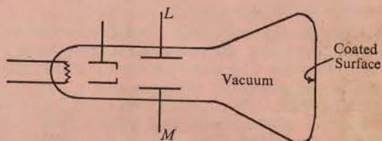
The diagram shows a tube suitable for producing a narrow beam of electrons and accelerating them so that they pass between two horizontal plates, *L* and *M*, before striking the far end of the tube which is coated with a fluorescent material.
