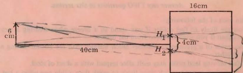
The diagram shows an illuminated arrow of length 6 cm placed 40 cm in front of a pinhole camera 16 cm in length having two small holes,  $H_1$  and  $H_2$ , 4 cm apart.
