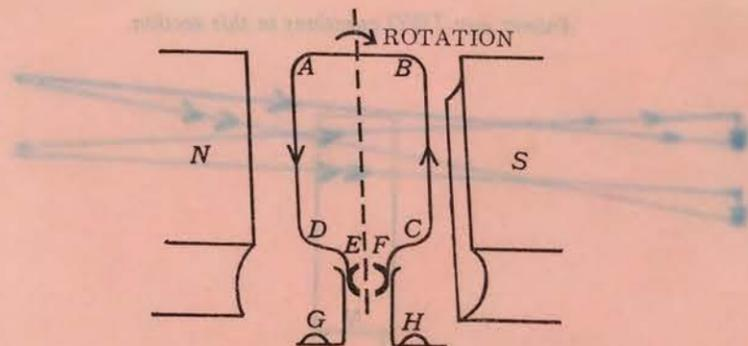
(i) The above is a simplified diagram to show the structure and action of a simple d.c. motor. Explain, briefly:
