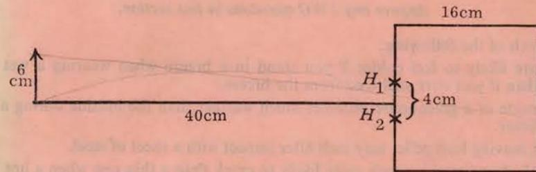
The diagram shows an illuminated arrow of length 6 cm placed 40 cm in front of a pinhole camera 16 cm in length having two small holes,  $H_1$  and  $H_2$ , 4 cm apart.
