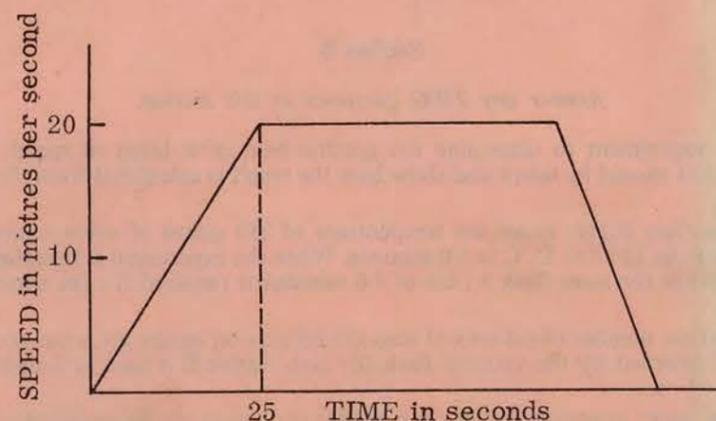
The graph shows the motion of a car which accelerates uniformly from rest to a speed of 20 metres per second in 25 seconds and is brought to rest from that speed with a uniform retardation of 400 cm per second<sup>2</sup> on a level unimpeded straight road. If the total distance travelled is 1 km, determine:
