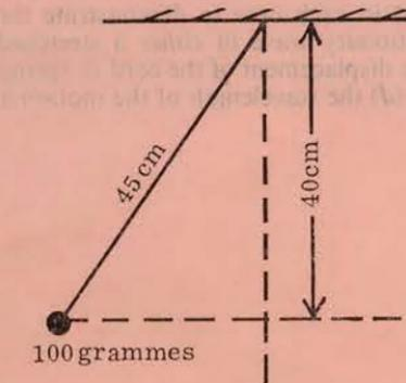
A small metal sphere of mass 100 grammes is suspended from a rigid support by a light string of length 45 cm. The sphere is then drawn aside, keeping the string taut, until its centre is 40 cm vertically below the supporting beam, as shown.
